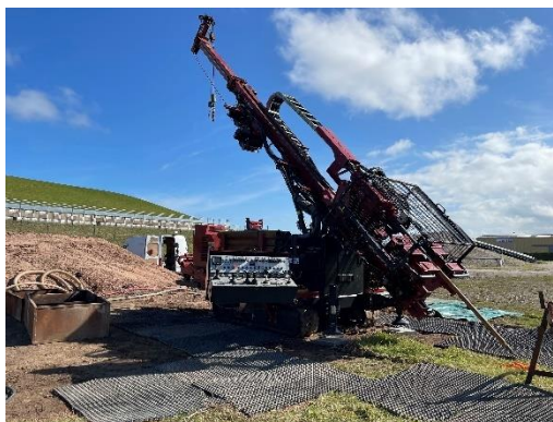
Figure 2-2 Photographies carottage d'investigation
